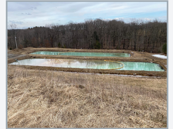
An acid-mine sludge pond in central Pennsylvania. A byproduct of coal mining, such sites may be rich with critical minerals. Credit: Provided by Sarma Pisupati
