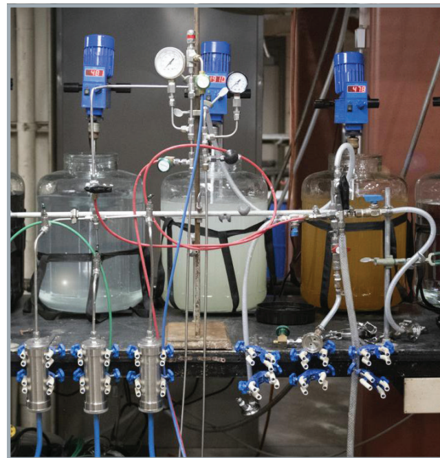
Experimental set-up in Sarma Pisupati's lab for extracting and separating critical minerals from acid mine drainage. Credit: Patrick Mansell
